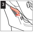
Open the lock-off opposite of the vehicle buckle by press down on the lock-off's tab.
